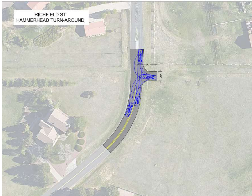
Figure 1: Proposed turn-around location on Richfield St, south of Hinsdale Ave, on the Chenango Bridle Path
