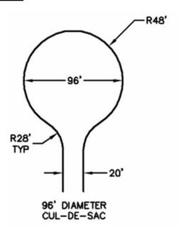
A cul de sac consists of a paved road with one end open to traffic and one permanently closed by a vehicle turn around. Per Arapahoe County standards, a minimum diameter of 96 feet is required.
