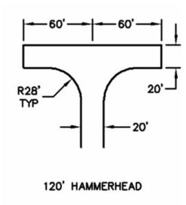
Paved road with one end open to traffic and one permanently closed by a vehicle turn around. Per Arapahoe County standards, a minimum length, perpendicular to the traveled path, of 120 feet is required.
