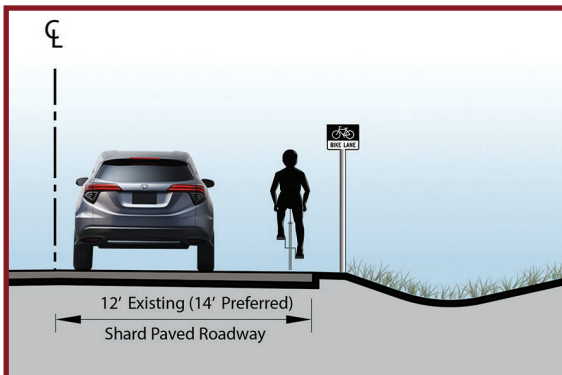
Figure 29: Typical Bike Route (shared road) Cross Section
